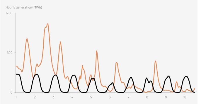
Source: AESO (2021). Note: This figure shows wind and solar generation in Alberta in 2021 over a 10-day period in July, showing the complementarity of these sources: solar generation is highest mid-day while wind generation is highest at night.
